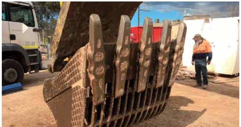
Sieve buckets fitted with K VX Penetration teeth are used for ripping out concrete footings, then loading the material into tipper.
